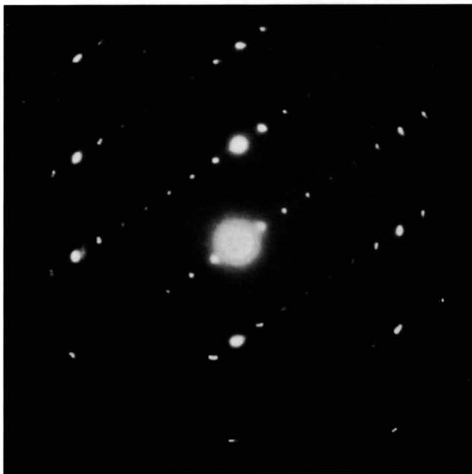
Fig. 2. (1\bar{1}0) reciprocal-lattice plane which corresponds to \{112\} or \{110\} in NaCl and b.c.c. types of structures respectively.
